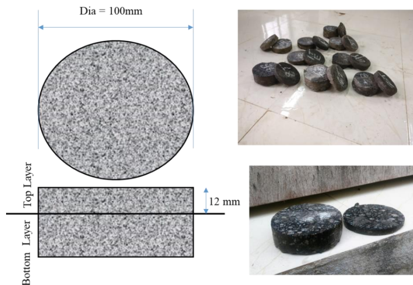
Figure 4.3 Schematic and actual photo of the sliced field core sample
