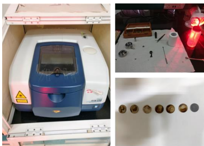
Figure 4.13: FT-IR Setup, sample preparation and samples
