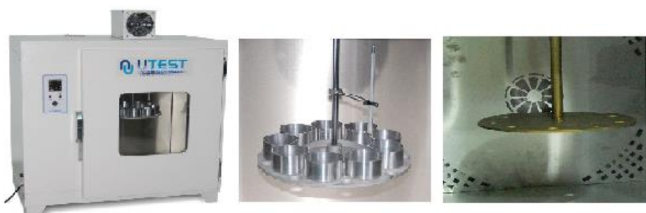
Figure 2.2: Thin Film Oven Test Apparatus (Controls-group, 2019)
