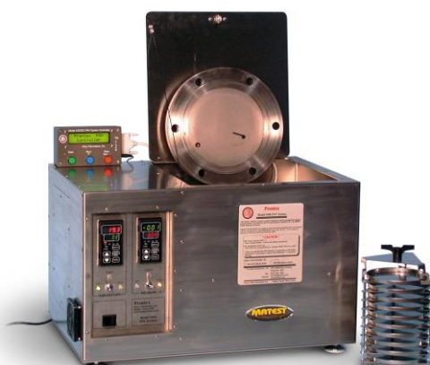
Figure 2.6: Pressure Aging Vessel (PAV) (Pavement Interactive 2019)
