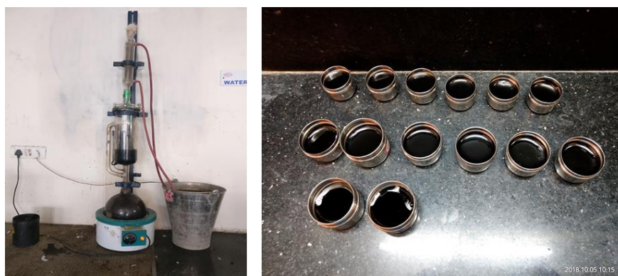
Figure 4.9: Soxhlet extractor and extracted bitumen samples
