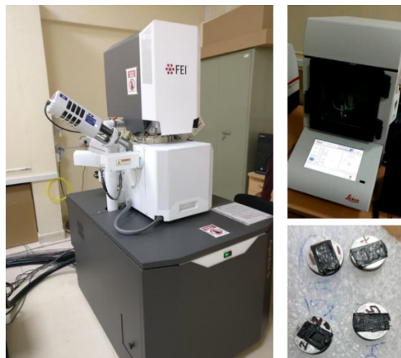
Figure 4.15: Field Emission Scanning Electron Microscope and samples
