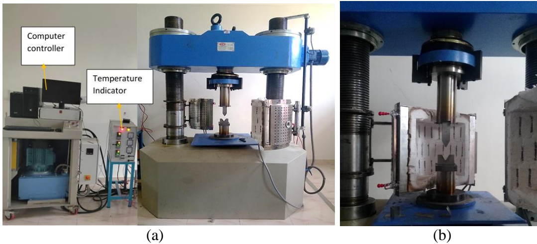
Figure 5.1 (a) Compression testing machine and (b) Heating split furnace
