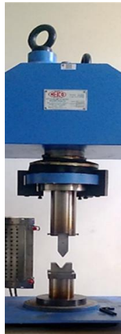
Figure 5.3 Loading of punch and die on CTM
