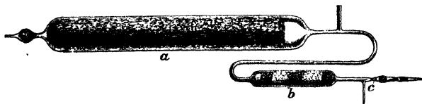
FIG. 30—MORLEY'S PALLADIUM-TUBE FOR WEIGHING HYDROGEN.
