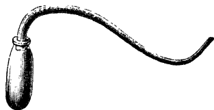
FIG. 37—STOPPERED FLASK USED BY PRIESTLEY IN PREPARING “VITRIOLIC ACID AIR” (Sulphur Dioxide).
