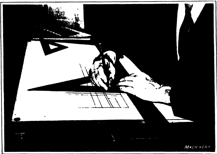
Fig. 15. Drawing a Vertical Line by using T-square and Triangle
