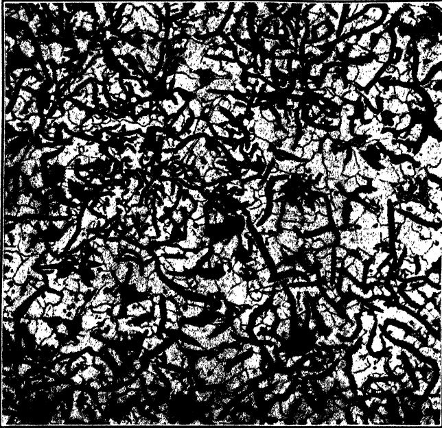
FIG. 92.—GRAY CAST IRON (A.S.T.M. CLASS 20B), ETCHED WITH 3 PER CENT NITAL, \times 100
