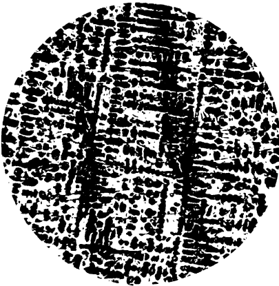
FIG. 219.—White Iron before annealing. Etched. \times 50 Dias. (Cementite and pearlite.)
