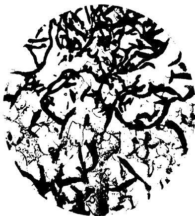
FIG. 214.—Annealed Cast Iron, 1-in. Section, heated for 1 hour at 820^{\circ} C. and air cooled. Etched. \times 200 Dias. (Ferrite, graphite, and phosphide eutectic.)
