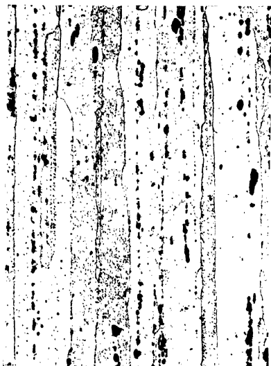
FIG. 254.—Longitudinal Section of “Duralumin B” extrusion. \times 200 Dias.
