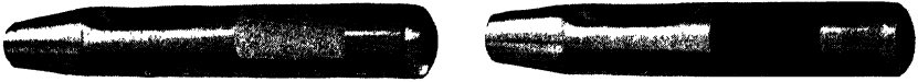
FIG. 97.—Indicating Paint. When 235^{\circ}\text{C} . is reached the original white colour of Thermindex Colour E.104 changes to dark grey. (Courtesy—Messrs. J. M. Steel and Co., Ltd.)
