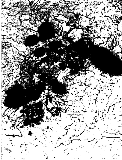
FIG. 284.—Gas cavities in mild steel weld. 50 Dias.
