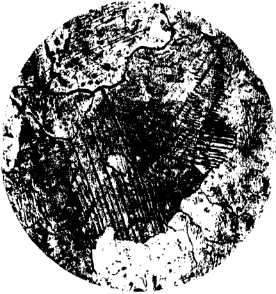
FIG. 237.—Cold-worked 70/30 Brass, showing presence of strain lines. \times 100 Dias.
