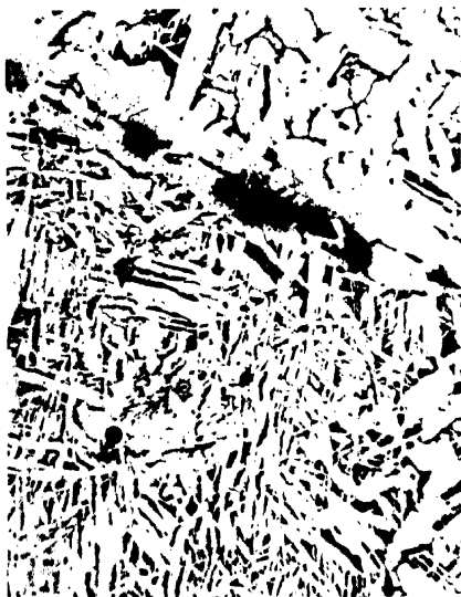
FIG. 281.—Lack of fusion and entrapment of oxide along fusion face of mild steel weld. \times 100 Dias.
