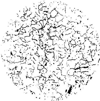
FIG. 230.—Structure near the surface of a Whiteheart Malleable iron casting. Etched. \times 100 Dias.
