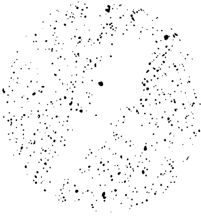
FIG. 242.—85 5 5 5 Gunmetal in unetched condition, showing free lead finely dispersed. \times 50 Dias.
