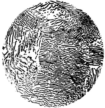
FIG. 142.—Steel containing 0.85 per cent carbon at higher magnification showing laminated structure of pearlite. \times 500 Dias.
