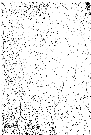
FIG. 199.—18/8 Chromium-Nickel Stainless Steel. As Cast. \times 100 Dias.
