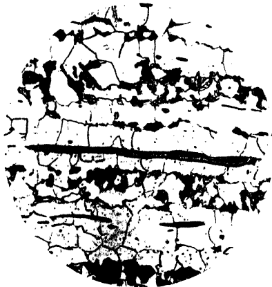
FIG. 190.—Free-Cutting Steel containing approx. 0.2 per cent sulphur. Note elongated sulphide in direction of rolling.
