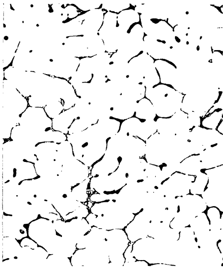
FIG. 251.—Duralumin as cast. Etched 30 secs. in 12½ per cent NaOH, \text{CuAl}_2 shows black and \alpha(\text{MnSi}) outlined and unattacked. \times 350 Dias.
