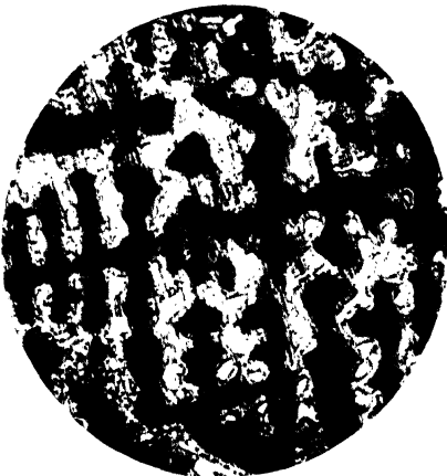
FIG. 244.—Phosphor Bronze. 88.5 Cu, 11 Sn, 0.5 P. Etched. \times 100 Dias.
