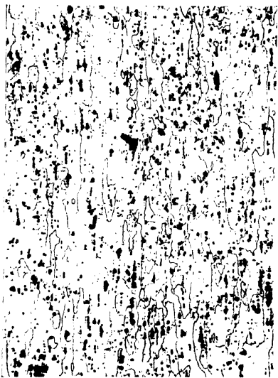
FIG. 253.—“Duralumin B” sheet. Longitudinal section. \times 100 Dias.
