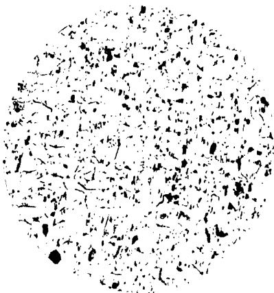
FIG. 205.—Fine Graphite in Cast Iron (Inoculated Type), Unetched. \times 50 Dias.
