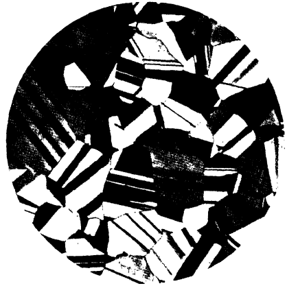
FIG. 238.—Cold-worked and annealed 70/30 Brass, showing twinned crystals. \times 50 Dias.
