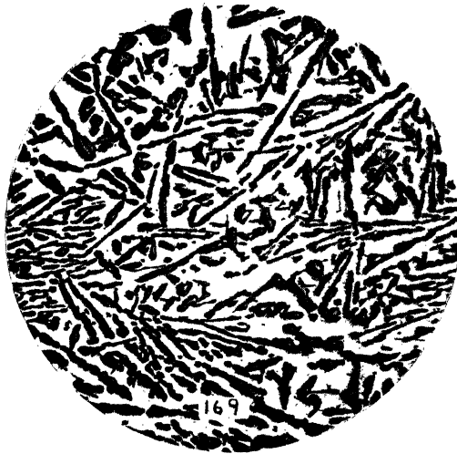
FIG. 256.—Sand-cast 12 per cent Silicon-Aluminium Alloy. Unmodified. Almost eutectic composition. \times 100 Dias. (Courtesy—Messrs Light Alloys Ltd.)
