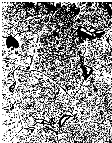
FIG. 255.—“Y” Alloy Solution treated and then precipitated for 450 hours at 285° C. During the extended treat- ment the precipitate, which is nor- mally ultramicroscopic, is easily visible at the magnification of 500 Dias.
