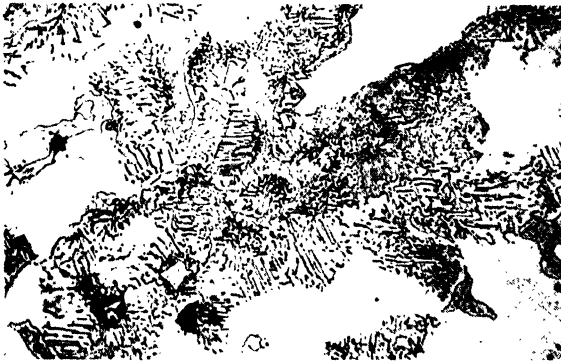
Fig. 6-4. "Vitallium" (H.S. 21) furnace cooled from 1300° C (2375° F). Etched with 6 per cent aqua regia. Magnification 250 \times . (After Badger and Sweeney)
