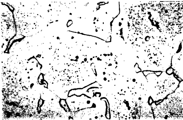
Fig. 3-8. C-Mo steel of the same general analysis as that in Figure 3-6 after a service life at 593° C (1100° F) of 30,000 hrs. Magnification 1000 \times . (After Miller, Golaszewski, and Smith)
