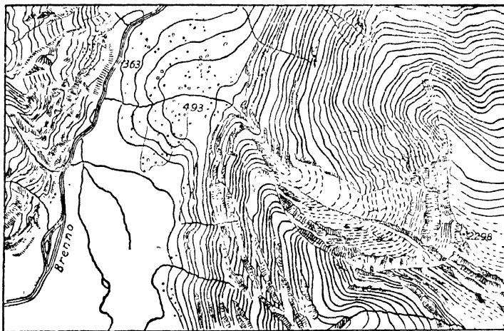
FIG. 44.—The Biasca torrent (scale 1 : 75,000, from the Swiss map on 1 : 50,000), showing the catchment basin, the channel, and the alluvial fan. A typical instance.
