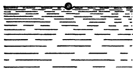
FIG. 6.—To show the depression of the surface of water when a needle is floated on it.
