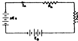
Figure 244-B — Equivalent circuit of three-electrode rectifier.
