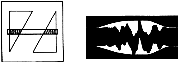
Figure 16-C — Push-pull Class A variable area.
