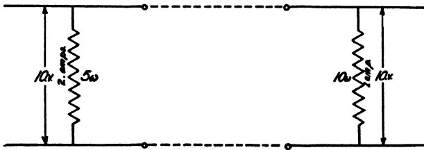
Figure 301 — Voltage and current ratios may be used when calculating db loss or gain, only if measured in equal resistances.
