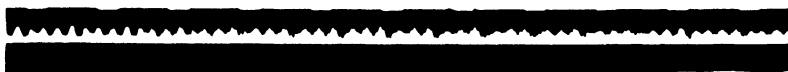
Figure 26-B — A single envelope variable area recording of the speech wave of Figure 26-A.
