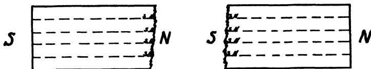
Figure 275 — When a bar magnet is broken, each piece becomes a magnet.
