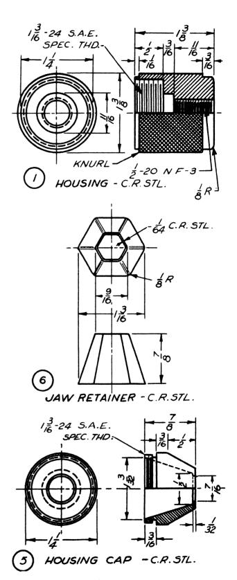
Fig. 188—DETAIL DRAWING OF DRILL CHUCK PARTS
