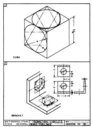
Fig. 116—isometric constructions (problems 1 and 2)
