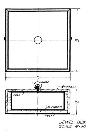
Fig. 65—ASSEMBLY SECTION DRAWING OF JEWEL BOX
