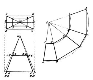
Fig. 127—DEVELOPMENT OF A PARTIAL PYRAMID
