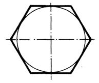
Fig. 112—constructing a hexagon outside
