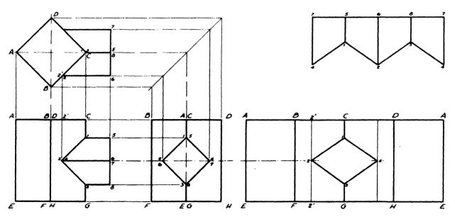
Fig. 137—INTERSECTION AND DEVELOPMENT OF TWO PRISMS
