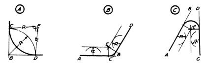
Fig. 108—ARCS TANGENT TO STRAIGHT LINES
