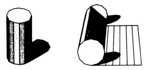
Fig. 129—cylinder represented with flat sides
