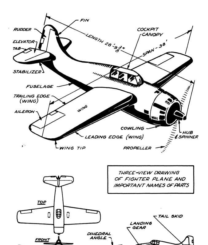
Fig. 224—A PICTORIAL AND A THREE-VIEW DRAWING OF A MODEL PLANE
