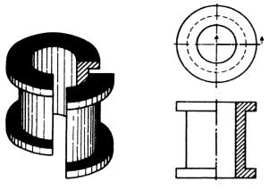
Fig. 63—HALF-SECTION DRAWING OF SPOOL
