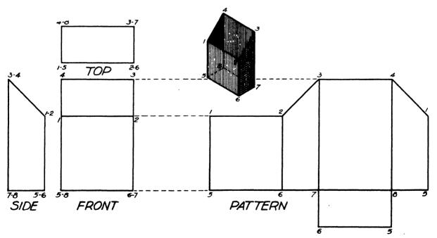
Fig. 122—Drawing and pattern for a matchbox holder
