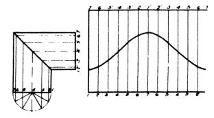
Fig. 132—DEVELOPMENT OF A TWO-PIECE ELBOW
