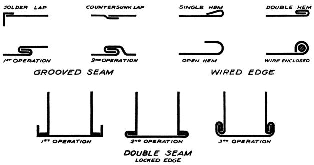
Fig. 120—metal seams and edges
