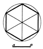
Fig. 110—CONSTRUCTING A HEXAGON WITH T SQUARE, TRIANGLE, AND COMPASS
