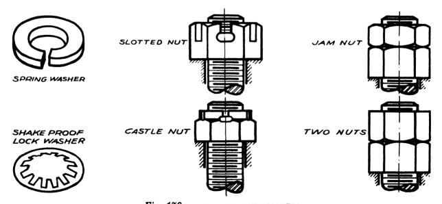
Fig. 170—Lock nuts and washers
