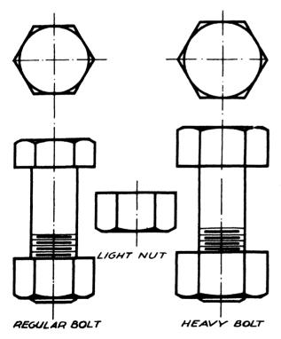
Fig. 164-standard bolts and nuts
