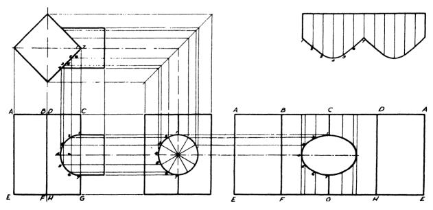
Fig. 138—Intersection and development of a cylinder and a prism
