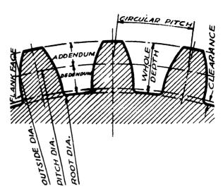
Fig.~201—names of gear parts
