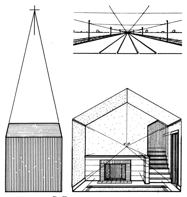
Fig. 77—one-point perspective drawing
