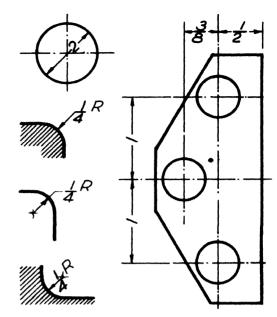
Fig. 46—DIMENSIONING CIRCLES AND ARCS
