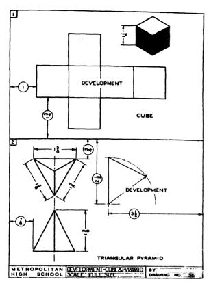
Fig. 143—DEVELOPMENT OF A CUBE AND A PYRAMID (PROBLEMS 1 AND 2)
