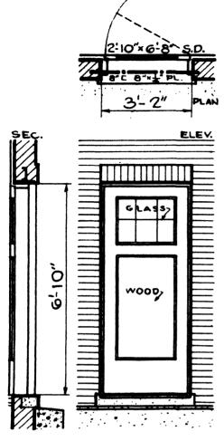
Fig. 245—Door in Masonry
