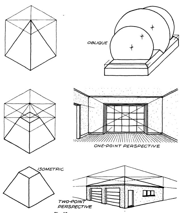
Fig. 83—FREEHAND PICTORIAL DRAWING
