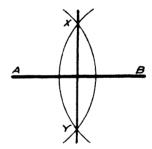
Fig. 98—BISECTING A LINE WITH A COMPASS
