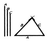
Fig. 106—constructing a triangle from three lines
