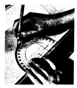
Fig. 6- MEASURING AN ANGLE WITH THE PROTRACTOR
