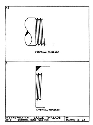
Fig. 206—LARGE THREADS (PROBLEMS 1 AND 2)
