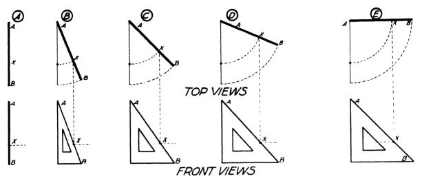
Fig. 123-THE TRUE LENGTHS OF LINES
