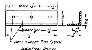
Fig. 228—RIVET DIMENSIONING
