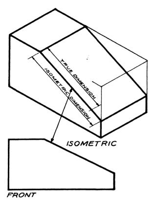
Fig. 80—nonisometric lines
