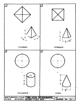
Fig. 68—TWO-VIEW ORTHOGRAPHIC DRAWING (PROBLEMS 1, 2, 3, AND 4)
