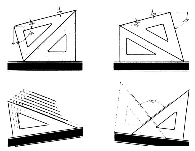
Fig. 39- Drawing lines at various angles
