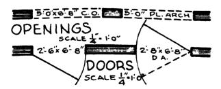
Fig. 249—doors and windows in interior frame walls
