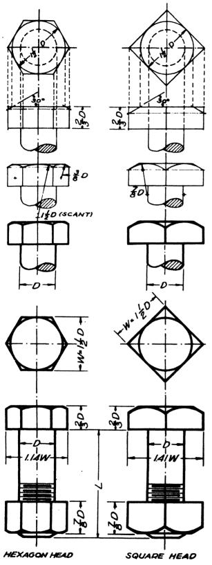
Fig. 166—standard bolt and nut proportions
