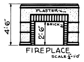
Fig. 25 --fireplace plan and elevation
