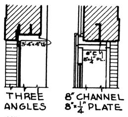
Fig. 247—LINTELS OF OPENINGS IN MASONRS
