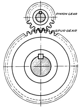
Fig. 200-A SPUR GEAR
