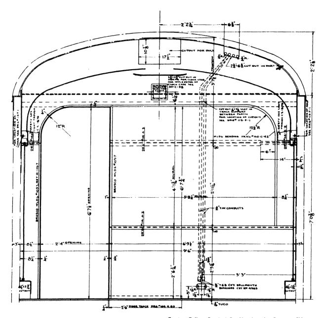
Courtesy Pullman-Standard Car Manufacturing Company, Chicago Fig. 190—DRAWING OF PARTITION AT END OF CAR IN FIGURE 189
