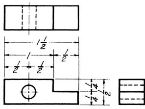
Fig. 37---comparison of the weights of lines
