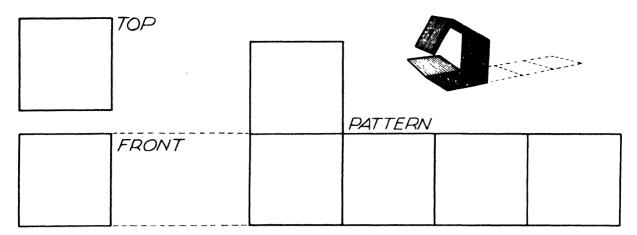
Fig. 121-—drawing and pattern for a small box
