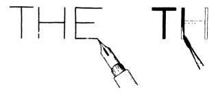
Fig. 19—single-stroke and built-up Letters
