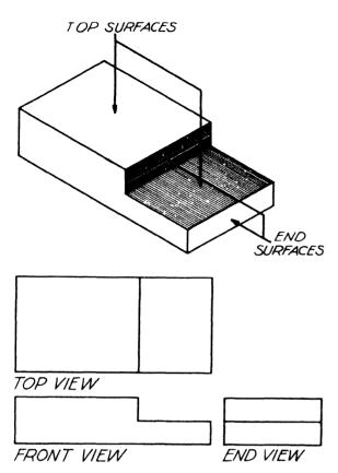
Fig. 57—orthographic drawing of cut
