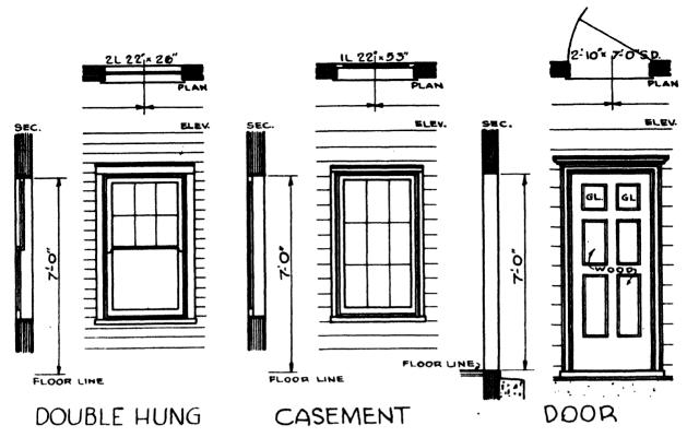
Fig. 248- doors and windows in exterior frame walls
