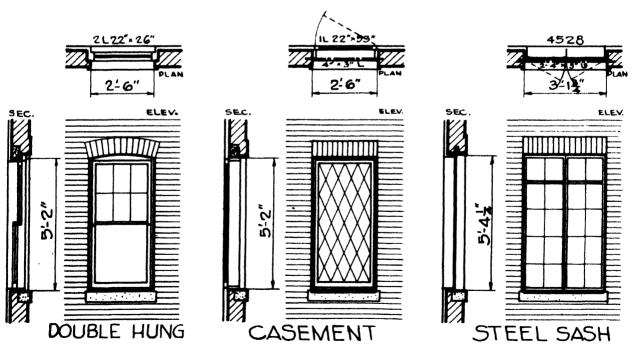
Fig. 244—windows in masonry
