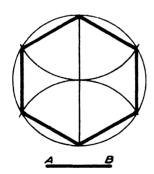
Fig. 111—constructing a hexagon with a Compass
