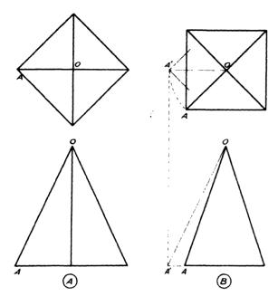
Fig. 124—the true lengths of edges on a pyramid
