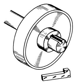
SKETCH SHOWS GIB-HEAD KEY TO FIT KEYWAY IN SHAFT AND WHEEL.
