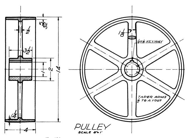
Fig. 186—A FULL SECTION AND A REVOLVED SECTION
