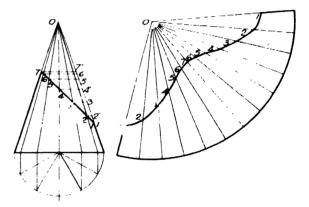
Fig. 134—DEVELOPMENT OF A PARTIAL CONE
