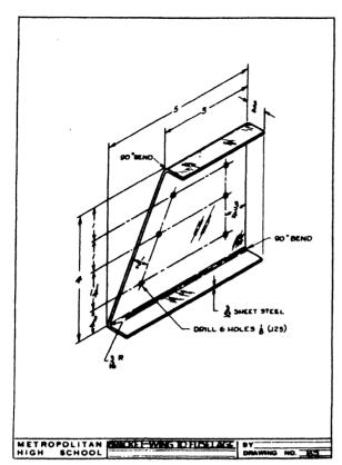
Fig. 230—BRACKET FOR FUSELAGE WING (PROBLEM)
