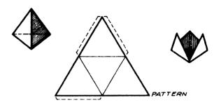
Fig.~119—seams on a pyramid
