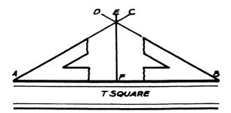
Fig. 99—BISECTING A LINE WITH TRIANGLE AND T SQUARE
