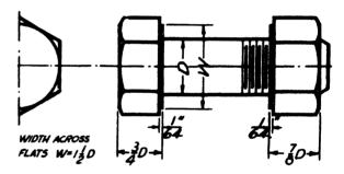
Fig. 165—A WASHER-FACED BOLT AND NUT
