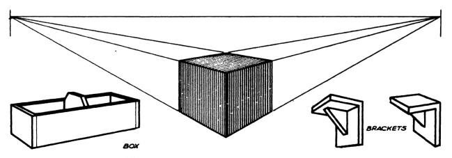
Fig. 81—Two-point perspective drawing
