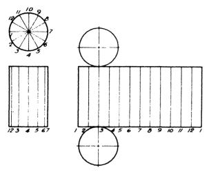
Fig. 130- - DEVELOPMENT OF A CYLINDER
