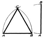
Fig. 105—constructing an equilateral triangle
