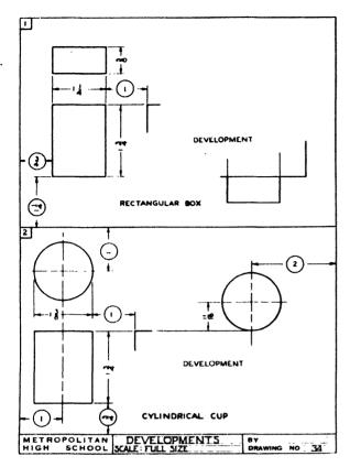
Fig. 141—DEVELOPMENT OF A BOX AND A CYLINDER (PROBLEMS 1 AND 2)
