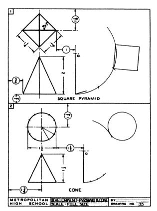
Fig. 142—DEVELOPMENT OF A PYRAMID AND A CONE (PROBLEMS 1 AND 2)
