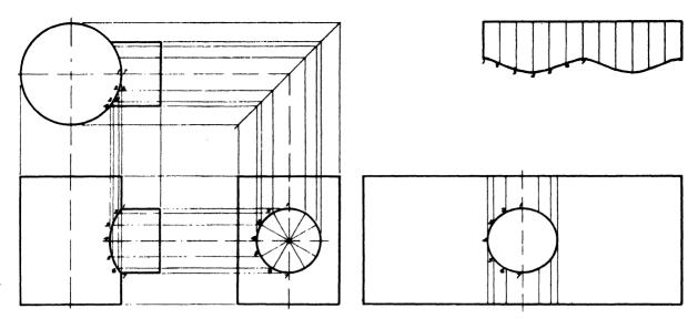
Fig. 139 - intersection and development of two cylinders
