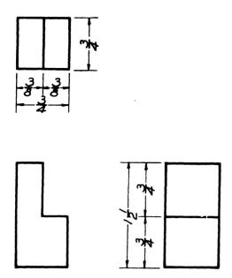
Fig. 44—DIMENSIONING A THREE-VIEW DRAWING
