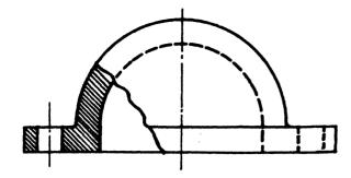
Fig. 185--A BROKEN, OR PARTIAL, SECTION
