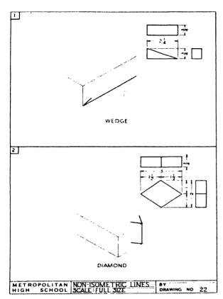
Fig. 90—nonisometric lines (problems 1 and 2)
