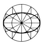
Fig. 113—THE CONCENTRIC-CIRCLE METHOD OF CONSTRUCTING AN ELLIPSE
