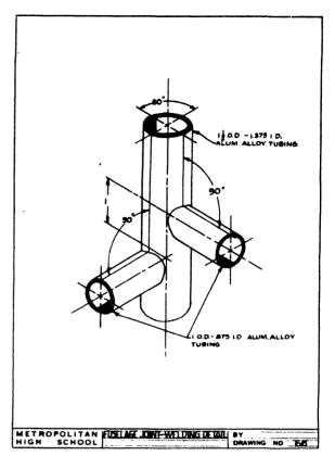
Fig. 231—welded joints in fuselage (problem)
