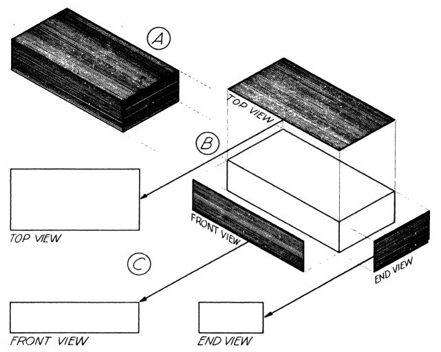
Fig. 56—orthographic drawing of block
