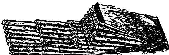
FIG. 13.—Sketch showing manner of placing logs in a typical log dam. ( Bull. 244, Office of Exper. Sta., U S Dept. of Agri.)
