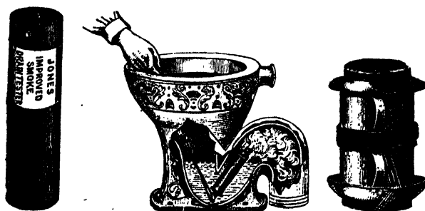
FIG. 84. SMOKE ROCKETS FOR DRAIN TESTING
