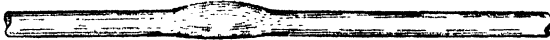
FIG. 78. SHOWING SWELLING IN LEAD PIPE CAUSED BY EXPANSION OF WATER DURING FROST
