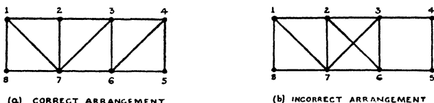
FIG. 81. CORRECT AND INCORRECT ARRANGEMENT OF BARS
