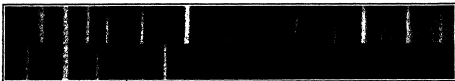
FIG. 434.—Powder photographs of the dimorphous forms of \text{FeS}_2 . Pyrite above, marcasite below.
