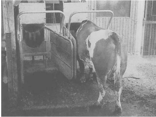
Figure 13.36 Output-related dosing of concentrated feed at an automatic feed booth for dairy cows. In the illustration the cow is identified by the transponder at its neck (reproduced by permission of Dr Georg Wendt, Landtechnischer Verein in Bayern e.V., Freising)
