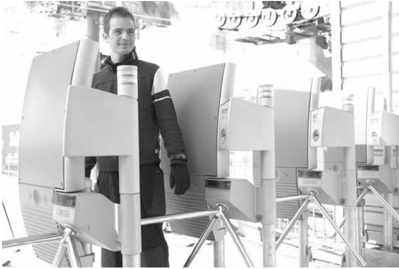
Figure 13.22 Contactless reader as access control and till device at a ski lift (reproduced by permission of LEGIC Identysystems AG, CH-Wetzikon)
