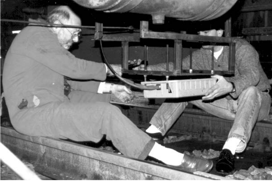
Figure 13.28 Fitting a read antenna for the Eurobalise onto a tractive unit (reproduced by permission of Siemens Verkehrstechnik, Braunschweig)
