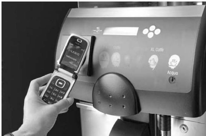
Figure 13.17 An NFC-enabled mobile phone with the corresponding payment application simulates a contactless credit or debit card (reproduced by permission of LEGIC Identysystems AG, CH-Wetzikon)
