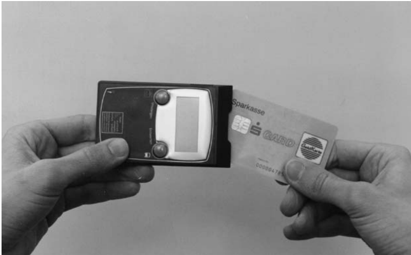
Figure 13.8 The contactless FlexPass of the district of Constance showing the GeldKarte and envelope (reproduced by permission of TCAC GmbH, Dresden)
