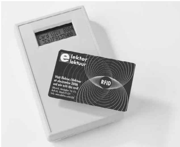
Figure 14.7 The reader in a plastic housing in stand-alone mode reads out the UID of a contactless smart card (reproduced by permission of Elektor, http://www.elektor.com )
