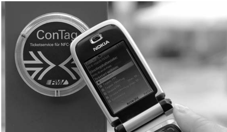
Figure 13.15 The RMV-ConTag – a passive transponder – can start the RMV-HandyTicket (mobile ticket) and the corresponding current timetable information. The mobile phone can load down the current data via an online connection (reproduced by permission of © RMV/Müller)
