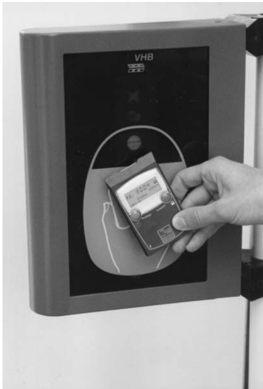
Figure 13.9 Contactless transaction using the FlexPass at a reader (reproduced by permission of TCAC GmbH, Dresden)
