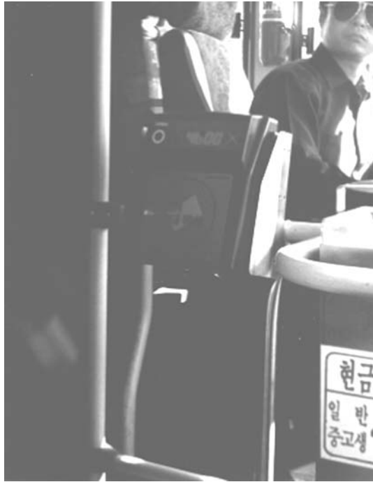
Figure 13.5 Reader for contactless smart cards at the entrance of a scheduled bus in Seoul (reproduced by permission of Klaus Finkenzeller, Munich)
