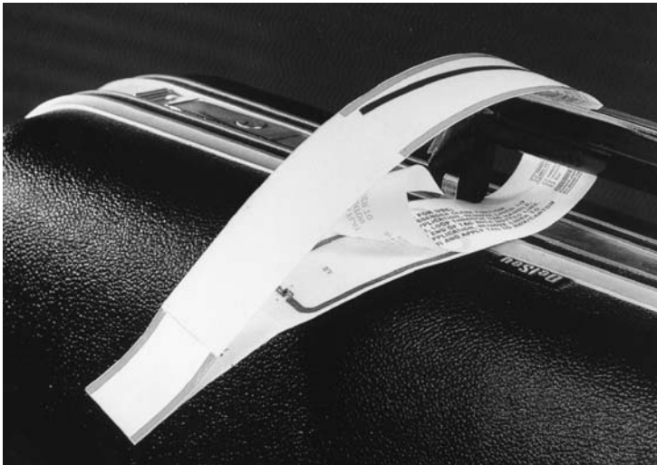
Figure 2.14 Smart label transponders are thin and flexible enough to be attached to luggage in the form of a self-adhesive label (reproduced by permission of i-code-Transponder, Philips Semiconductors, A-Gratkorn)
