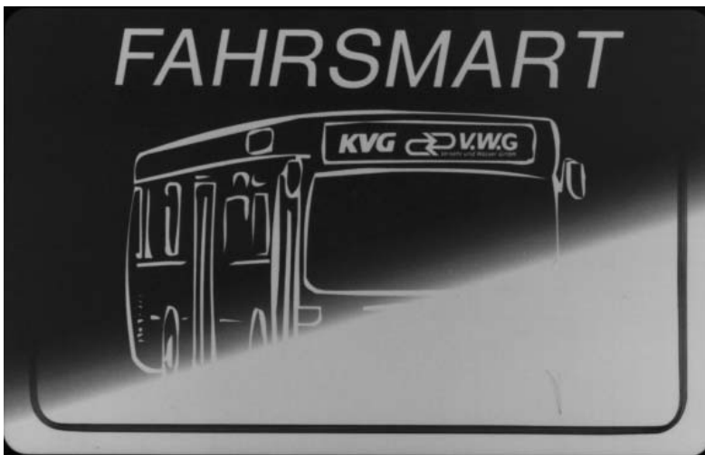
Figure 13.7 Fahrsmart II contactless smart card, partially cut away. The transponder coil is clearly visible at the lower right-hand edge of the picture (reproduced by permission of Giesecke & Devrient, Munich)
