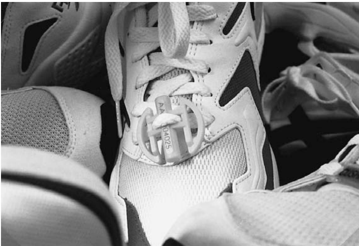
Figure 13.51 The ChampionChip transponder is fastened to the runner's shoe with the shoelace (reproduced by permission of ChampionChip BV, NL-Nijmegen)
