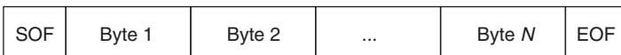
Figure 9.31 Structure of a message block (framing) made up of frame start signal (SOF), data and frame end signal (EOF)
