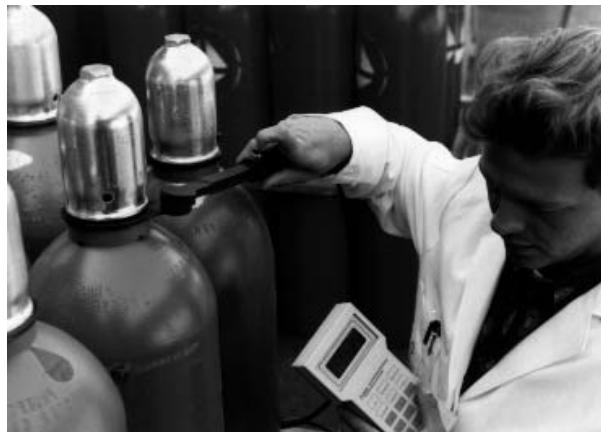
Figure 13.46 Identification of gas bottles using a portable reader. The reader (scemtec SIH3) is designed to function with transponders from different manufacturers (reproduced by permission of Messer Griesheim)
