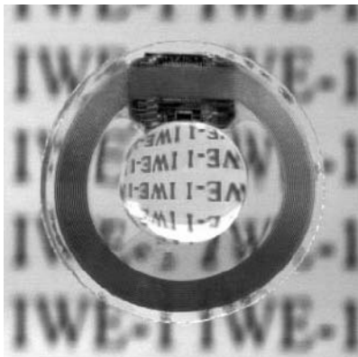
Figure 13.61 Transponder unit after casting into an artificial intraocular lens made of silicon (reproduced by permission of IWE1, RWTH Aachen, D-52074 Aachen)
