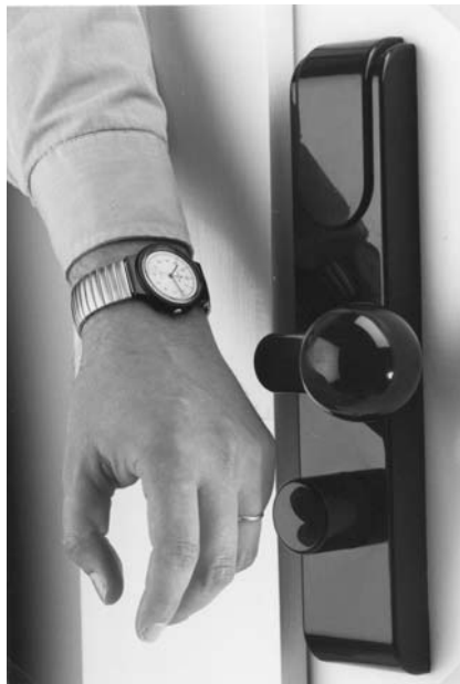
Figure 2.10 Watch with integral transponder in use in a contactless access authorisation system (reproduced by permission of Junghans Uhren GmbH, Schramberg)
