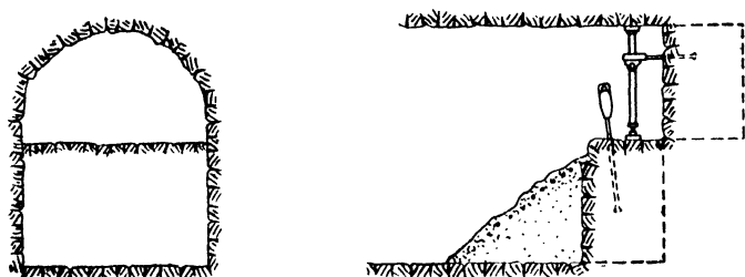
Fig. 269.—Heading-and-bench system. The bench is being drilled with hand sinker drills from the floor of the top heading.
