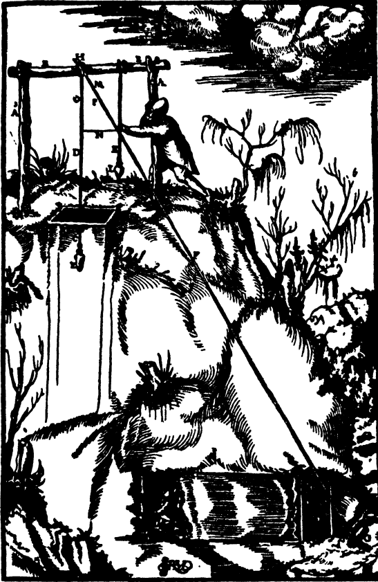
FIG. 3.—The early mine surveyor. Aligning a drainage tunnel to intersect a shaft by a system of similar triangles. A , upright forked posts; B , pole over the posts; C , shaft; D , first cord; E , weight of first cord; F , second cord; G , same fixed to ground; H , head of first cord; I , mouth of tunnel; K , third cord; L , weight of third cord; M , first side of minor triangle; N , second side of minor triangle; O , third side of minor triangle; P , the minor triangle. (From " De Re Metallica ," 1556.)
