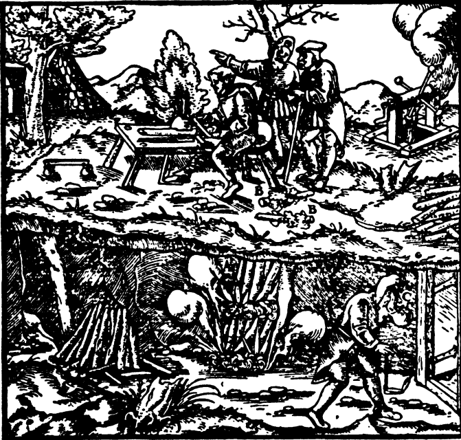
FIG. 1.—Breaking rock by fire-setting. The miner has just lighted a fire against the face and is retreating, holding his nose. The laborer on the surface is preparing "kindling sticks." A, kindled logs; B, sticks shaved down fan-shaped; C, tunnel. (From " De Re Metallica ," 1556.)
