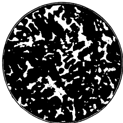
FIG. 165.—The white body is a eutectic surrounding the crystallites first formed.
