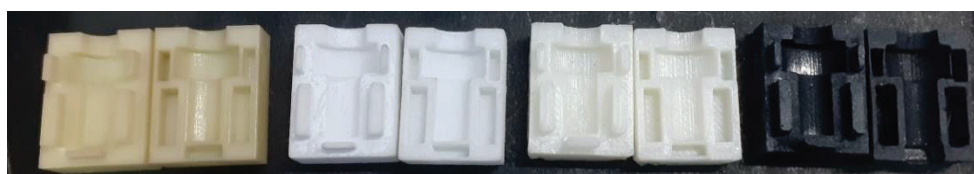
(a) Moulds printed through SLA, SLS, FDM and VC (left to right)
