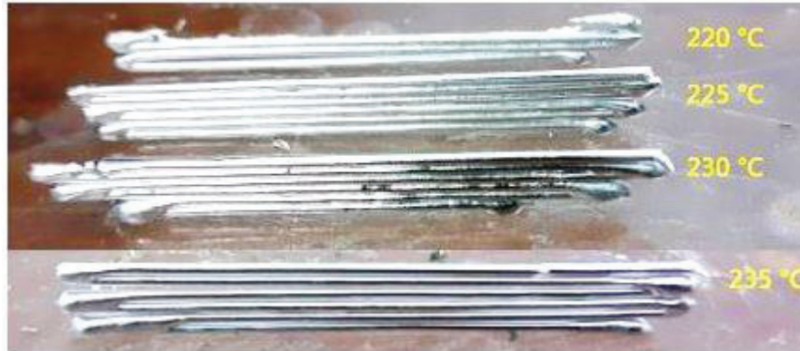
Figure 3.10: Six layers stacking at different temperatures and 90°C bed temperature
