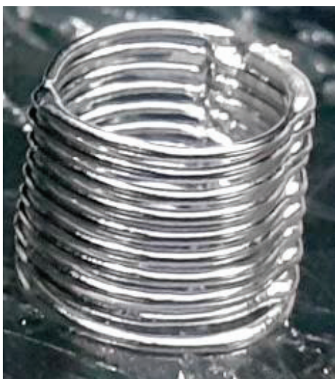
(a) Hollow circular strand of ten layers
