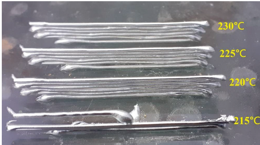
Figure 3.8: Six layers stacking at different temperatures and 90°C bed temperature
