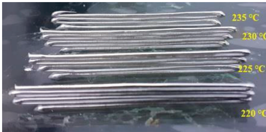
Figure 3.14: Six layers stacking at different temperatures and 90°C bed temperature
