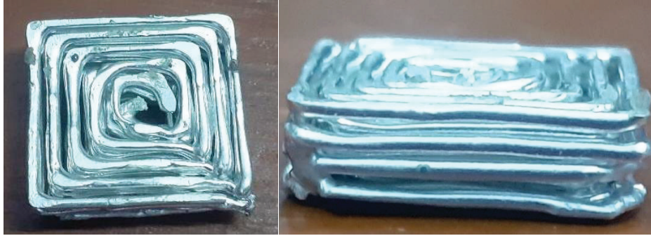
Figure 3.26: Cuboid profile (15.86 X 15.87 X 5.43 mm) deposited through extraction and dwell (top view-left, side view-right)
