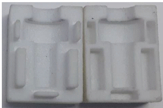
(c) SLS mould intact after repeated use
