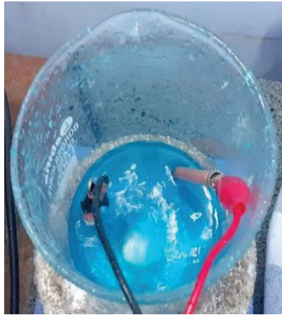
Figure 5.8: Whirling motion achieved using magnetic bead
