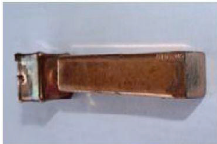
Figure 2.7: Electroplated profile after secondary metallization [101]
