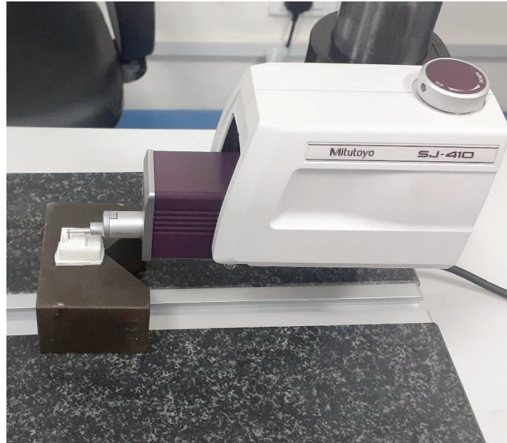
Figure 4.11: Surface roughness measurement
