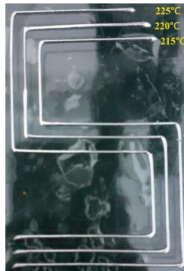
(b): Continuous deposition of Sn89Bi10Cu (60 mm/min) at different temperatures
