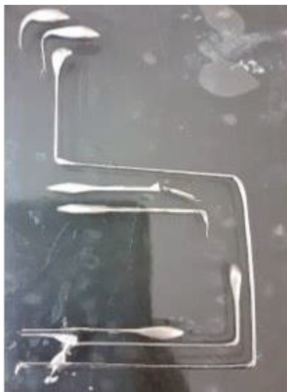
(a) Discontinuous deposition at high speed (> 100 mm/min)
