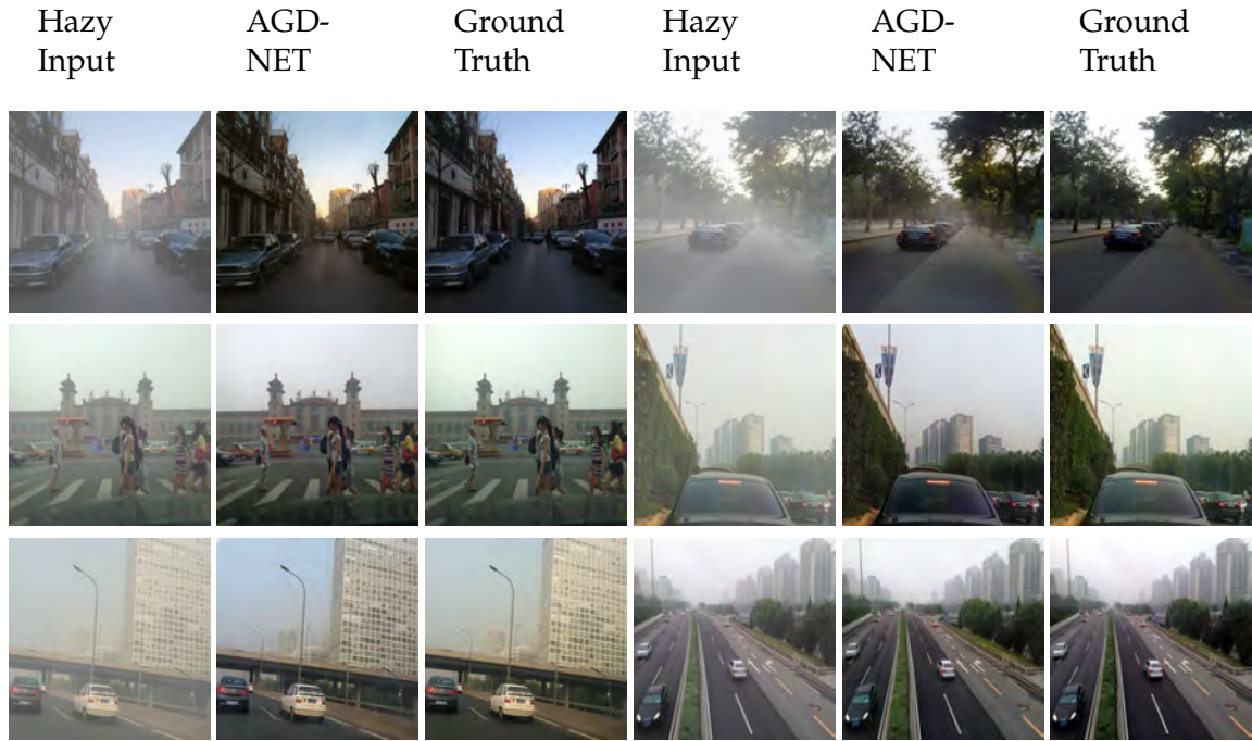
Figure 6.10: Visual comparison of the AGD-NET model’s generated results on the RESIDE- \beta SOTS Outdoor Dataset [9]
