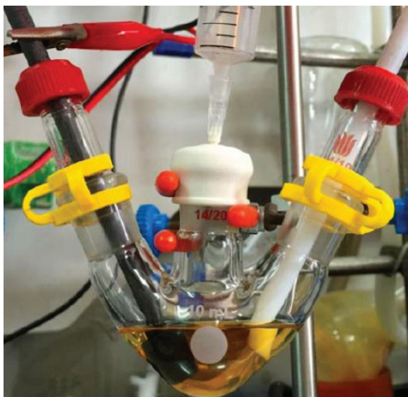
Figure 1.5 Undivided cell setup. Top left: Schematic representation; top right: Home-made; bottom left: Home-made; Commercially available electrasyn 2.0 from IKA
