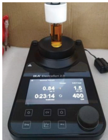
Figure 1.5 Undivided cell setup. Top left: Schematic representation; top right: Home-made; bottom left: Home-made; Commercially available electrasyn 2.0 from IKA
