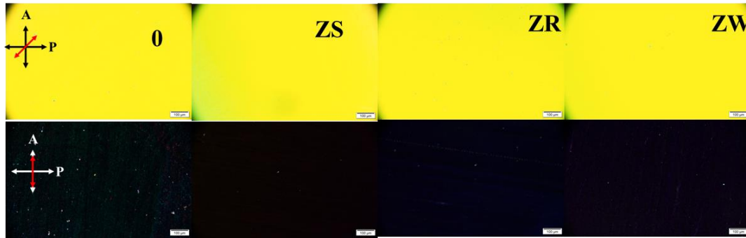
Figure 5-3 Optical textures of pure and 0.01 wt% ZnO nanocomposites of PCH5 observed between crossed polarizers under POM showing homogeneous alignment and no aggregation of nanoparticles in NLC.
