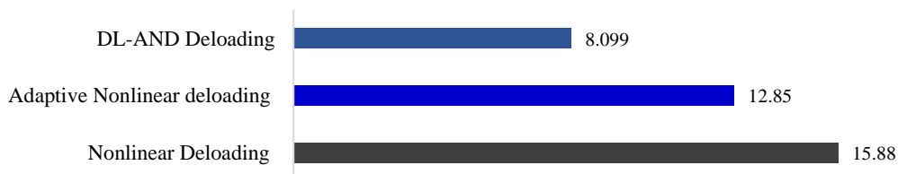
Fig. 6.11 Objective function ‘J’ with nonlinear deloading, nonlinear adaptive deloading and DL-AND strategy under FFOPID control structure
