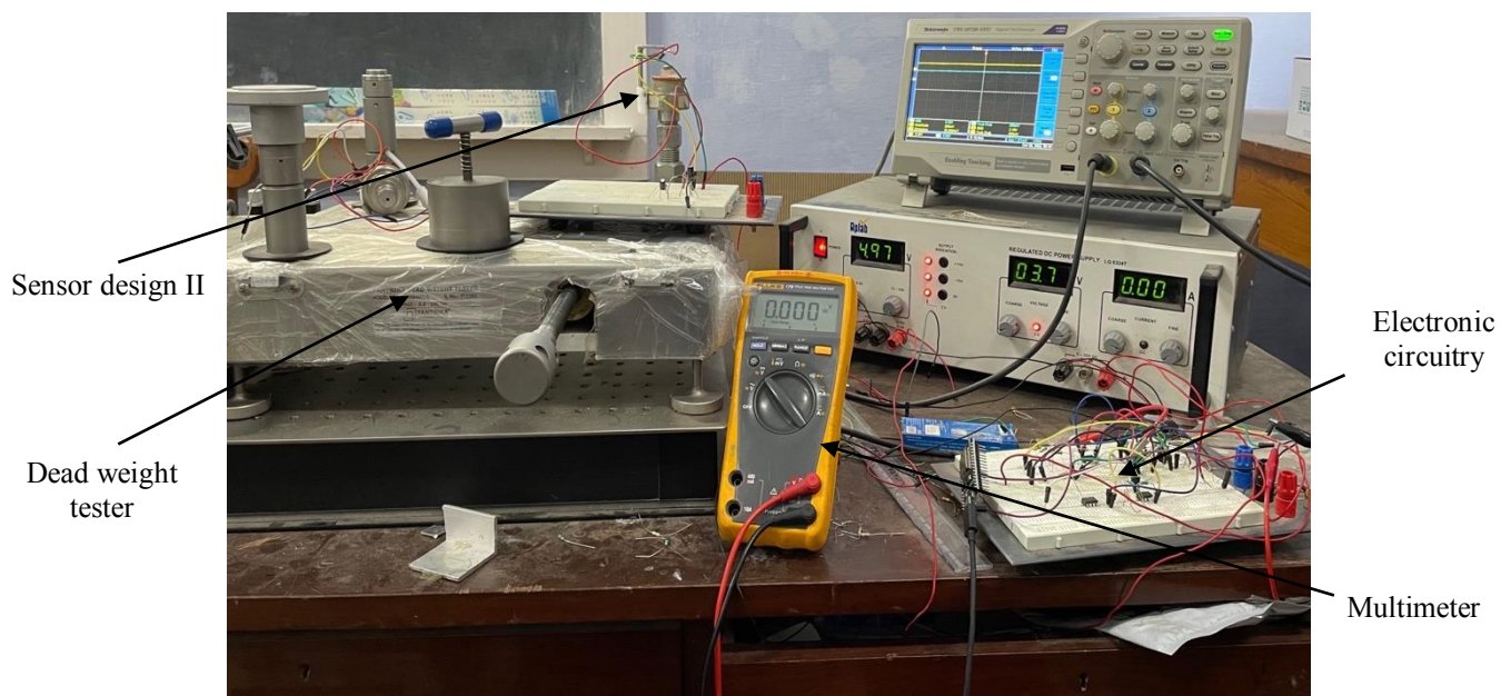
Fig. 5.10 Experimental setup of a wired transmitter for design II
