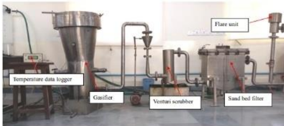
Fig. I.1 Photograph of downdraft gasifier set up
