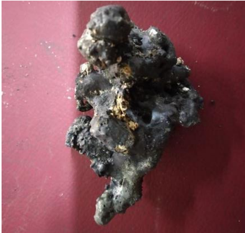
Fig. 5.32 Photograph of the fused clinker formation
