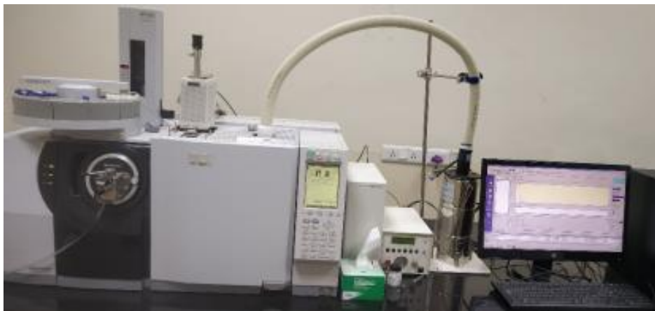
Fig. I.4 Photograph of Pyrolysis-gas chromatography-mass spectrometry set up
