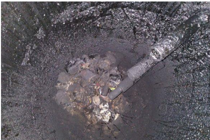
Fig 5.26 Picture of the inside of the gasifier for the oxy gasification of RDF pellets
