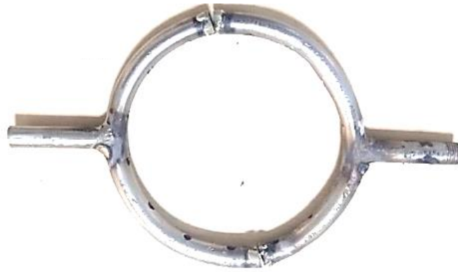
Fig. 3.3 Photograph of sparger
