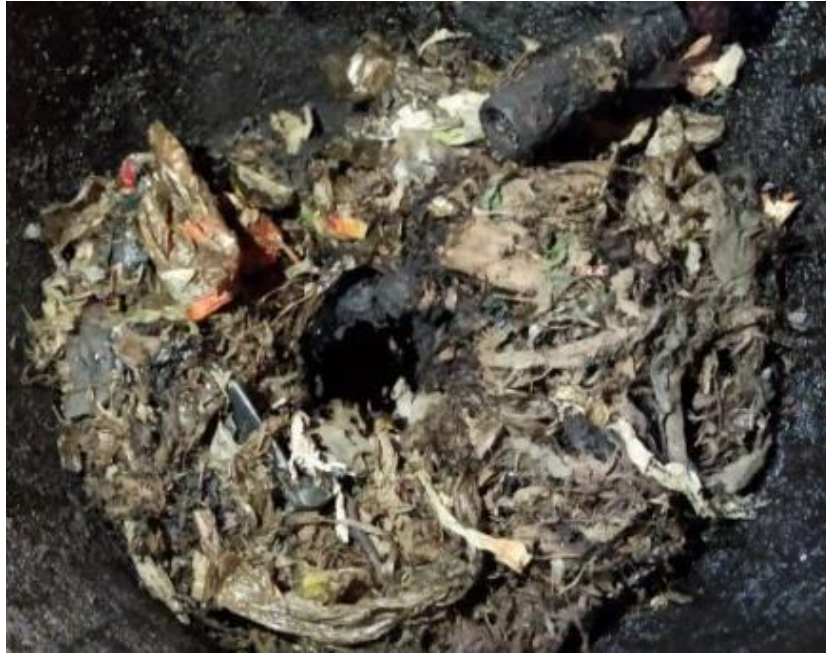
Fig. 5.24 Picture of the inside of the gasifier for the RDF fluff gasification
