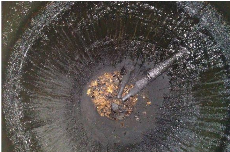
Fig. 5.28 Picture of the inside of the gasifier for the RDF pellet-biomass pellet mix (30:70) gasification
