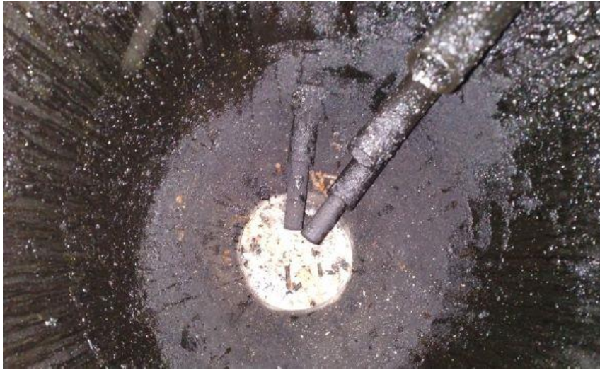
Fig. 5.27 Picture of the inside of the gasifier for the RDF pellet-biomass pellet mix (50:50) gasification
