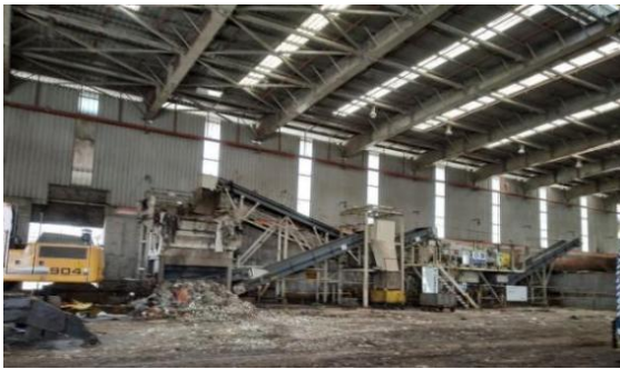
Fig. 2.12a AF shredder operation in a cement plant
