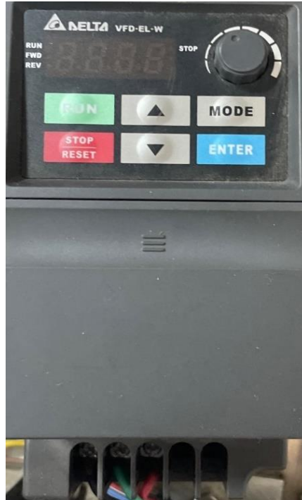
Figure 3.18 0.25 HP Variable frequency drive
