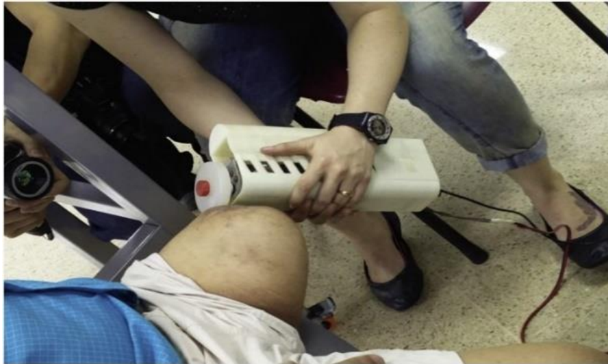
Figure 2.16 Handheld tribometer used for the measurement of COF at the residual limb [15]
