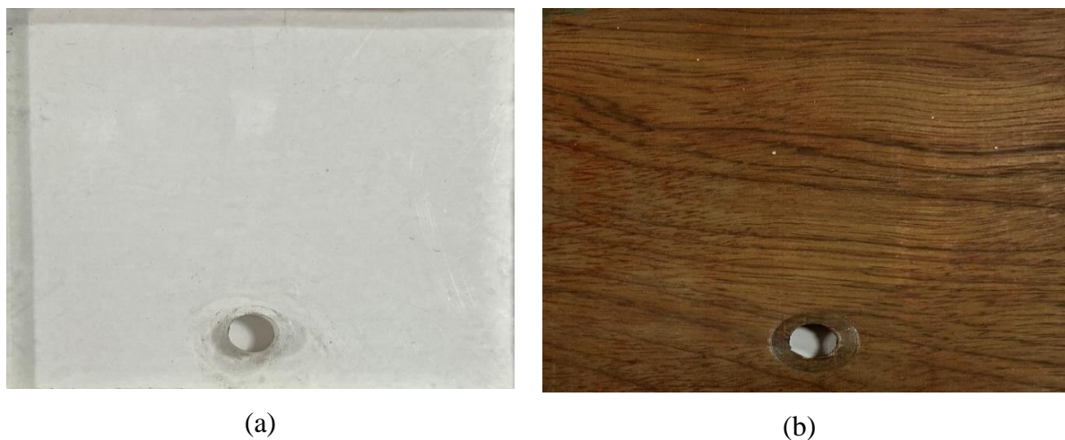
Figure 4.21 Fabricated plates used as test material (a) Acrylic and (b) Wood
