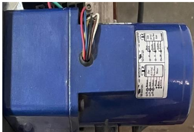
Figure 3.17 Phase 40-Watt Induction Motor
