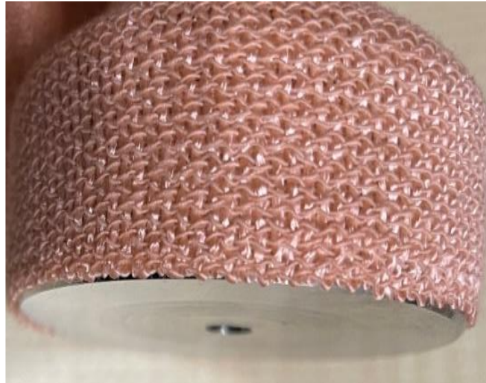
Figure 4.3 Wool mounted over the cylindrical probe
