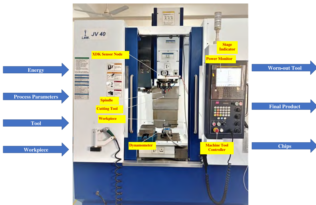
Figure 5.2 Physical world comprising of CNC vertical milling center with integrated sensor networks and devices; energy and material flow
