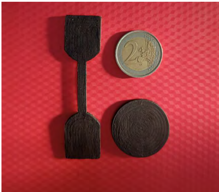
Figure 5.3. MWCNTs/PDMS composites for tensile and pressure sensor testing.
