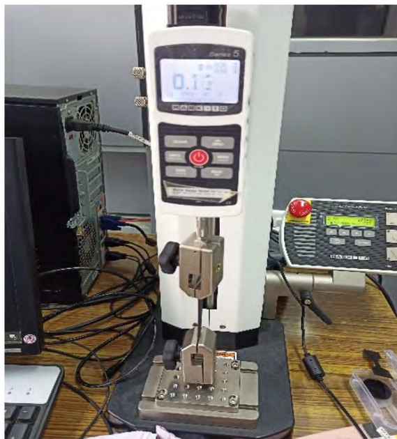
Figure 3.5. Mark-10 instrument setup for tensile testing.
