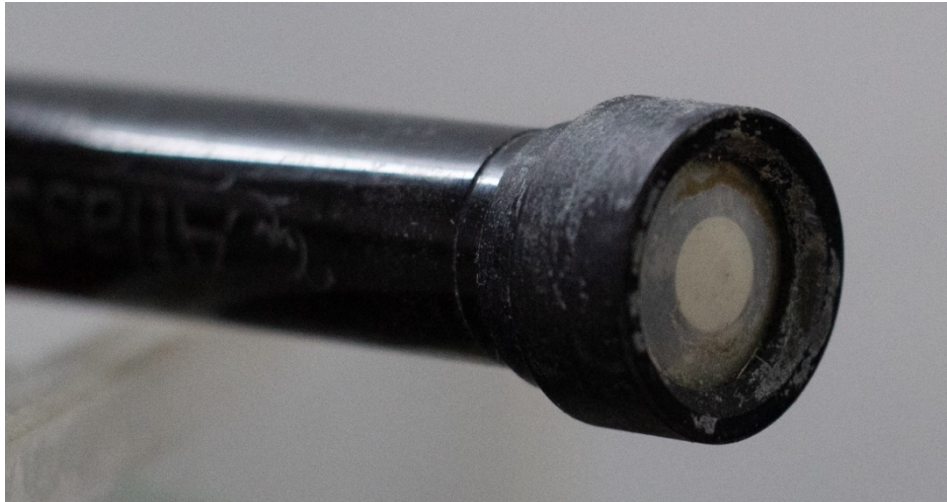
Figure 3. 8: DO electrode - detailed view of the interacting membrane
