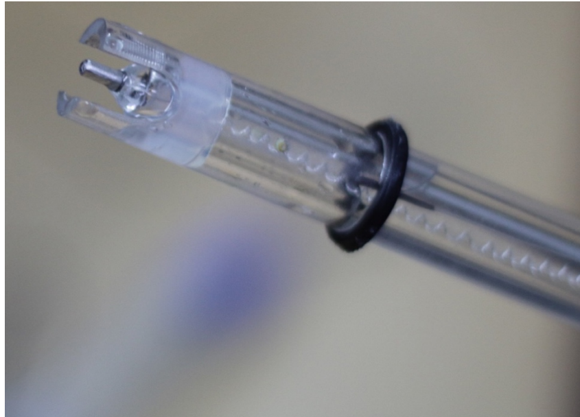
Figure 3. 6 : ORP electrode - detailed view of the interacting Pt Electrode
