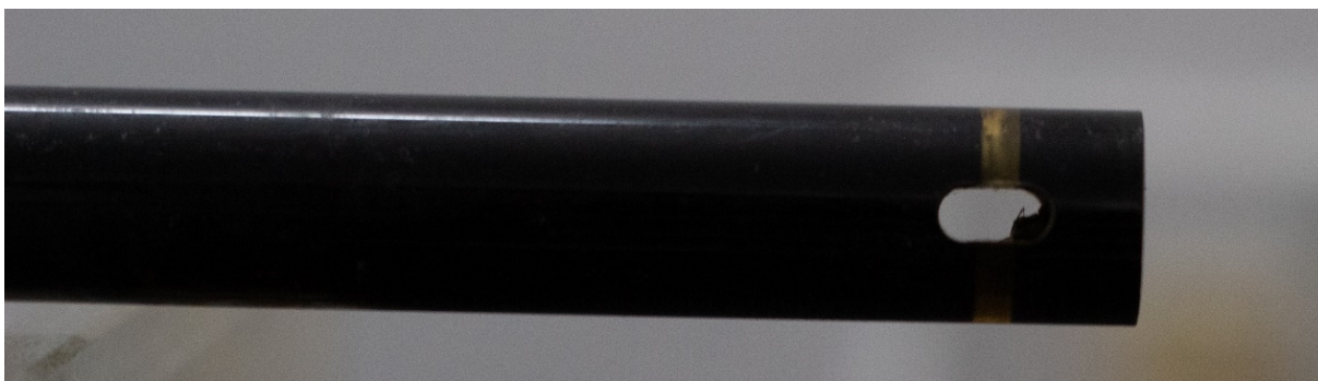
Figure 3. 11: EC electrode detailed view. The two plates between which the conductivity is measured are placed inside the eye-hole
