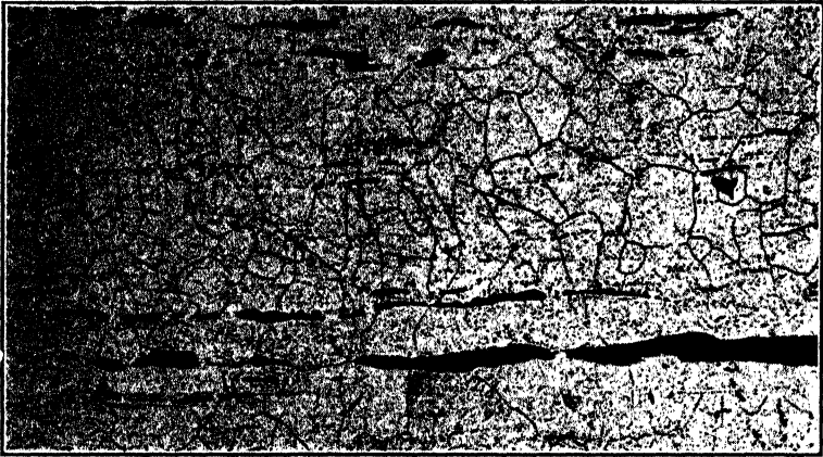
FIG. 11.—Magnified longitudinal section of a piece of wrought iron, showing the manner in which slag lines extend in the direction of rolling (Photomicrograph—longitudinal section \times 100 ).
