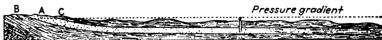
FIG. 131.—Transition of pervious water-bearing bed into close-textured impervious one. A, pervious stratum; B and C, impervious confining strata. (After Chamberlin.)
