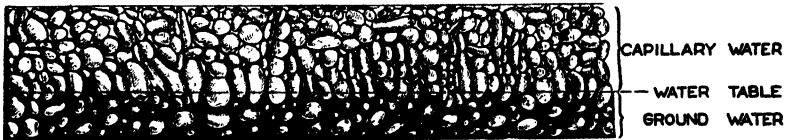
FIG. 5.—The capillary fringe. Capillary interstices near the base of the fringe are saturated; ground air appears in increasing amounts toward the top of fringe.
