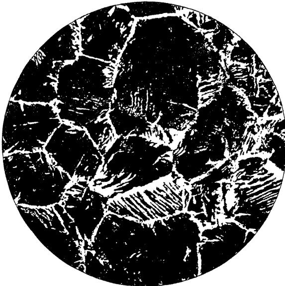
FIG. 60.—The same steel heated to 1050° for two hours and cooled in air. ( \times 100 .)
