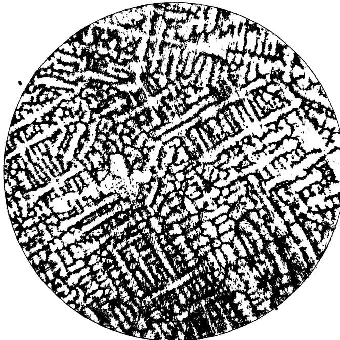
FIG. 67.—Brass cast in chill (70 per cent. Cu, 30 per cent. Zn). ( \times 75 .)
