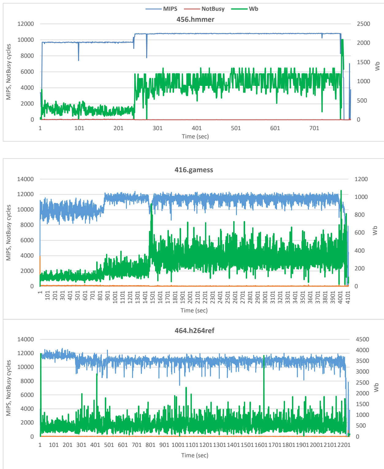
Figure 4.12: MIPS, NotBusy & Wb characteristics of core-benchmarks (456.hammer, 464.h264ref and 416.gamess)
