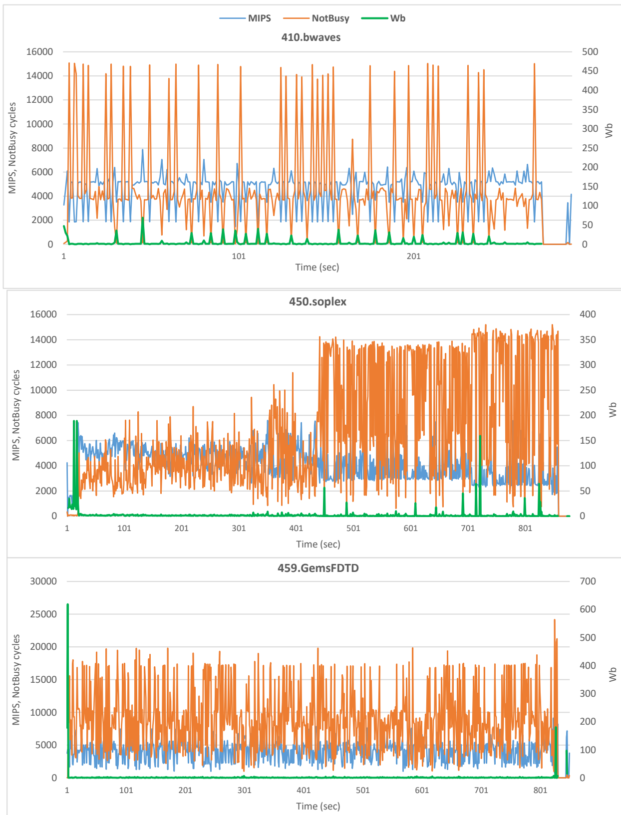
Figure 4.13: MIPS, NotBusy & Wb characteristics of memory-benchmarks (410.bwaves, 450.soplex and 459.GemsFDTD)
