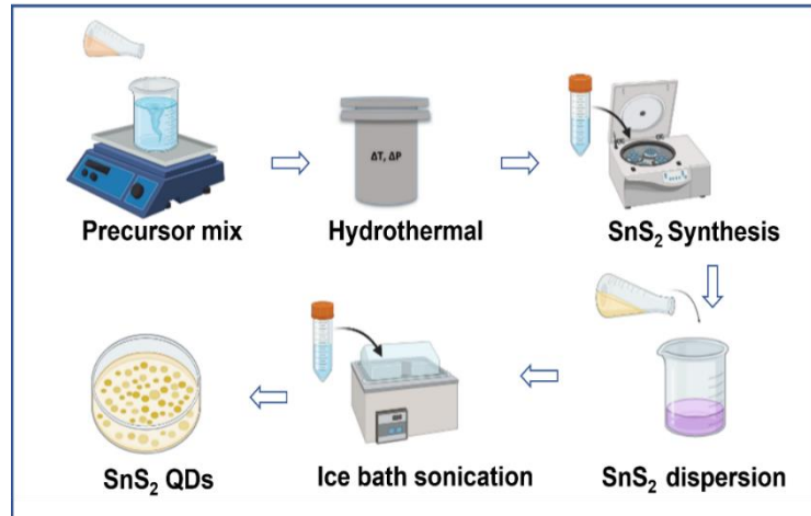
Figure S31: Schematic view of SnS 2 QDs synthesis.
