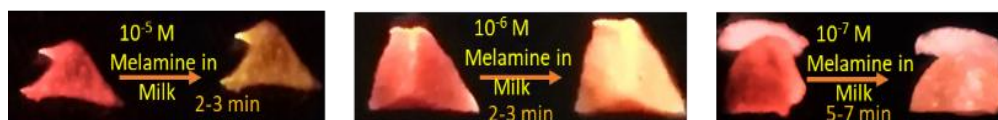
Figure 2.40 Acid-fumed ATHio4P polymer matrix with different shapes for melamine sensing in an actual milk sample
