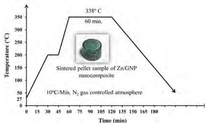
FIGURE 3.14: Sequence of the thermal procedure applied to sinter Zn/GNP nanocomposite pellets.
