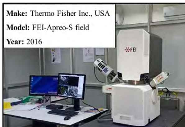
FIGURE 3.7: Field emission scanning electron microscopy (FESEM) attached with energy dispersive spectroscopy (EDS, Oxford Instruments).
