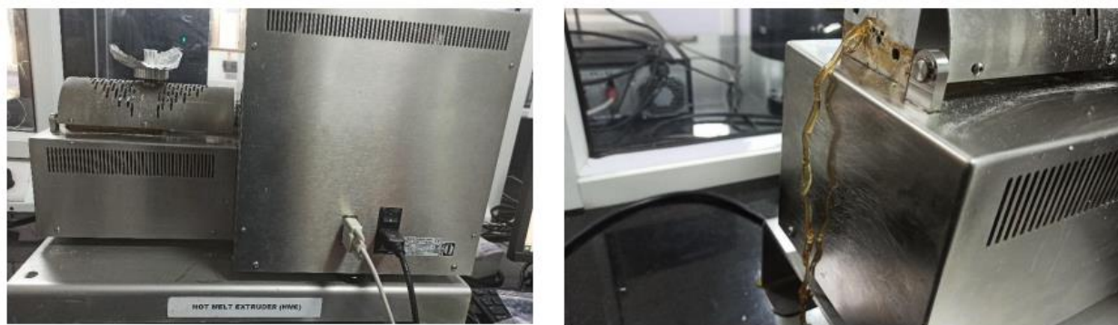
Figure 6.5. HME instrument for the preparation of ABTA SD
