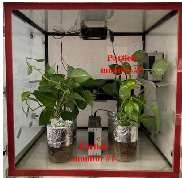
Figure A.5. Chamber with plants and two particle monitors to determine the well-mixed duration.
