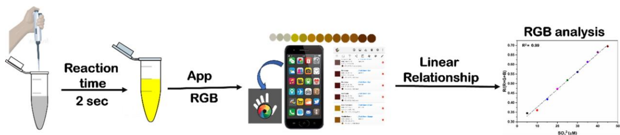
Figure 3B.25: Integration of the BPPyz with a smartphone
