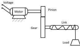
Q5b. What is the load applied on the link, if the change in resistance of strain gauge of resistance  $100 \Omega$  is found to be  $0.2 \Omega$ ? Take Modulus of Elasticity of the link material as 200 GPa and area of cross section is  $7.5 * 10^{-6} m^2$ . **3** M
