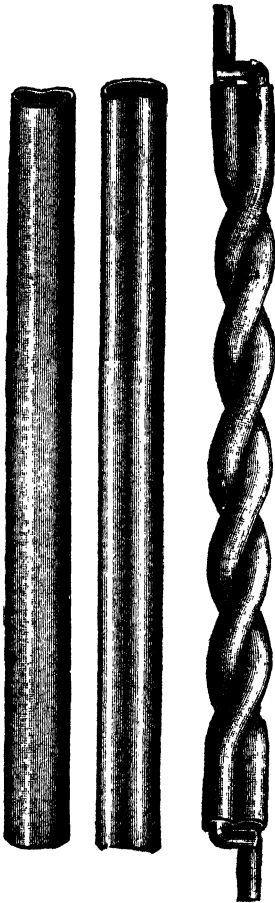
FIG. 18.—Type of joint for overhead conductors.
