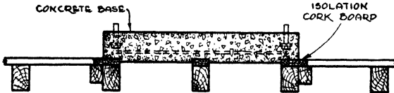
Fig. 6. Foundation—Mill Type Floor Construction
