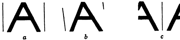
FIG. 16.12. Effect of Speed Difference (b) and Difference in Starting Point of Scanner and Recorder (c) on Appearance of Reproduced Picture (a).
