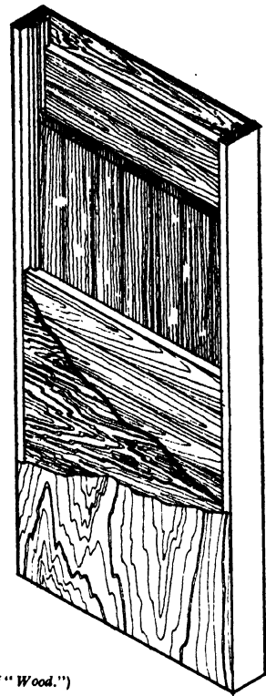
FIG. 202. Isometric drawing of RGC patented flush door which is of plywood construction.
