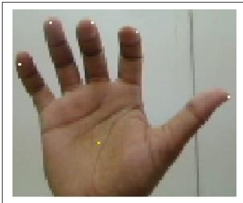
Figure 6.4: Fingertips and centre of palm detected in a real time system.
