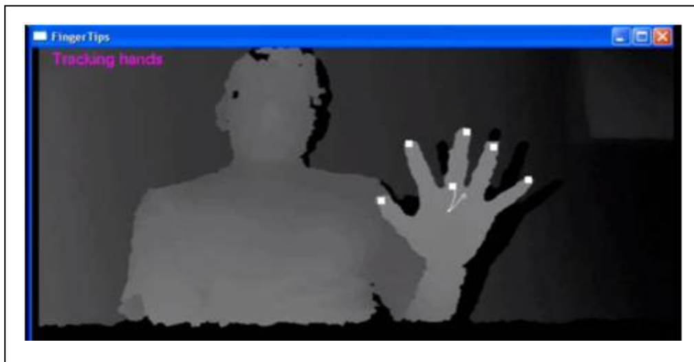
Figure 6.8: Result of fingertip detection in real time.
