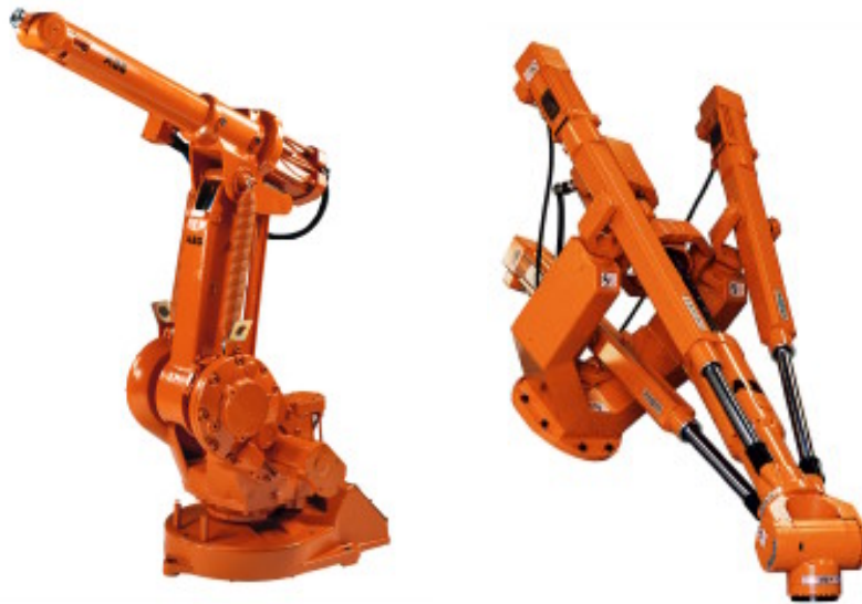
Fig. 3.1. A serial manipulator (left), the ABB IRB1400, and a parallel manipulator (right), the ABB IRB940Tricept.
