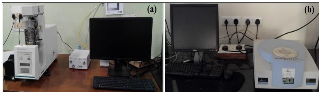
Figure 2.11: Photograph of (a) Shimadzu TGA-50 and (b) Perkin Elmer TGA-4000 TGA analyzers
