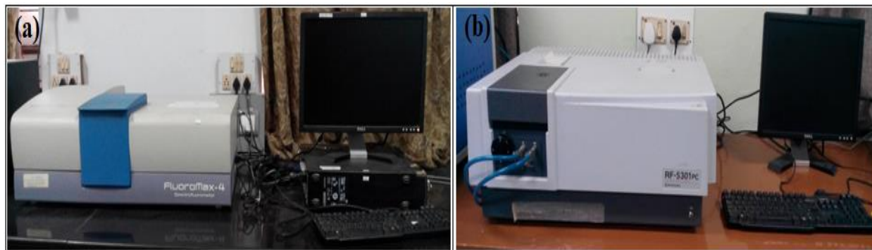
Figure 2.10: Photograph of (a) Horiba Jobin Yvon Fluoromax-4 and (b) Shimadzu RF-5301PC Spectrofluorimeters
