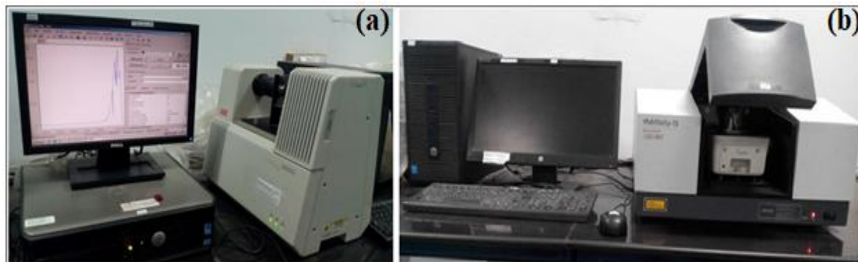
Figure 2.4: Photographs of (a) ABB Bomen MB-3000 and (b) Shimadzu IR Affinity-1S IR instruments
