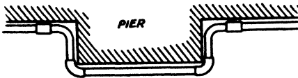
Fig. 16.—ONE METHOD OF FORMING A PASSOVER BEND, USING FITTINGS Not considered good practice.
