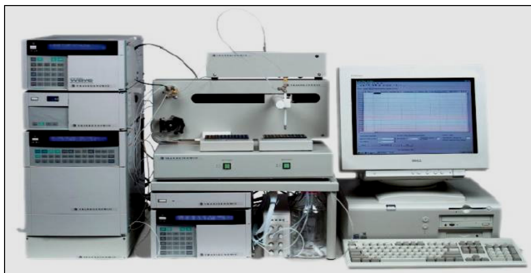
Figure 12:- Wave DNA Fragment Analysis System. The system from Transgenomics is exclusively used for separation of nucleic acids.
