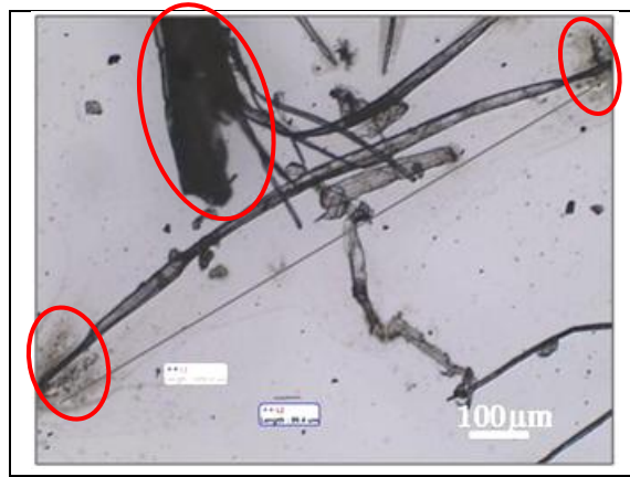
Fig 4.10: Stereomicroscopy image of whole bagasse pulp fibers pith. (The three red circles indicate glue like material which has resulted due to the degradation of pith cells at 165°C)
