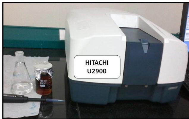
Fig 5.3: UV-Vis spectrophotometer used for black liquor analysis
