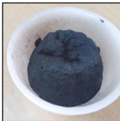
Fig 5.13: Retentate after incinerating in muffle furnace at 525°C
