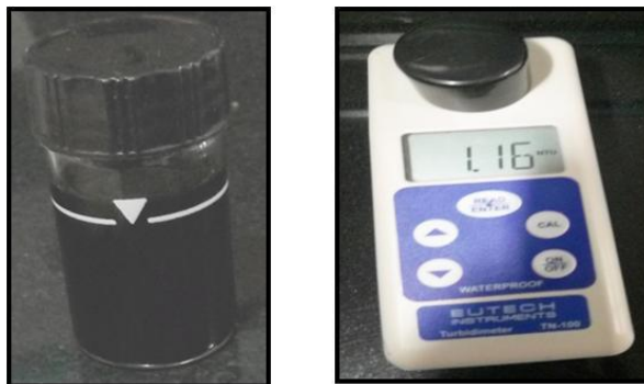
Fig 5.2: Black Liquor sample during turbidity measurement using Nephelometer
