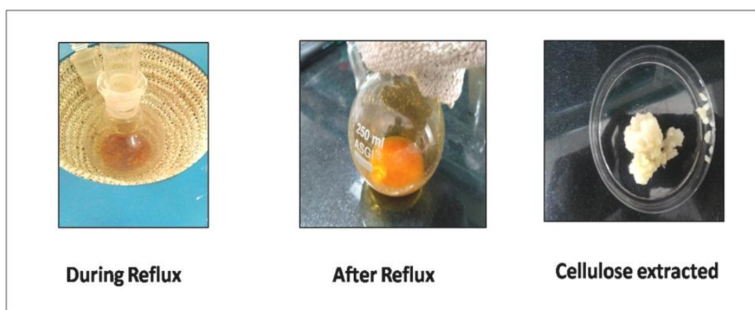
Fig 4.5: Bagasse pulp samples during and after cellulose test
