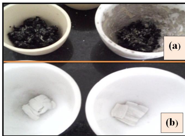
Fig 3.5: (a). Ash obtained from pulp (b). Ash obtained from wood chips.
